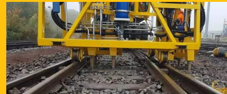
Tamping in the switch area
